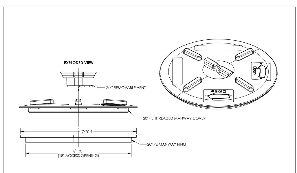
\*ALL EXTERNAL PIPING MUST BE INDEPENDENTLY SUPPORTED. \*ONLY BASE FITTINGS TO BE LEFT INSTALLED AT TIME OF SHIPMENT PER SII PROCEDURE. ALL DIMENSIONS ARE IN INCHES, NOMINAL, & SUBJECT TO CHANGE WITHOUT NOTICE. ALL DIMENSIONS ON ROTATIONAL MOLDED PARTS ARE SUBJECT TO A  $\pm$  3% TOLERANCE.
