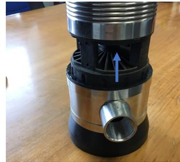
**Step-4:** Ensure alignment of intake will avoid any obstructions.
