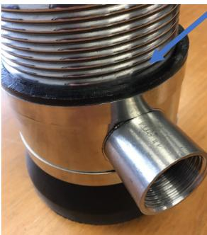
**Step-5:** Using weight of PUMP push into rubber cup to first radius as shown.
