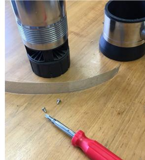
**Step-2:** Remove filter screen from PUMP.
