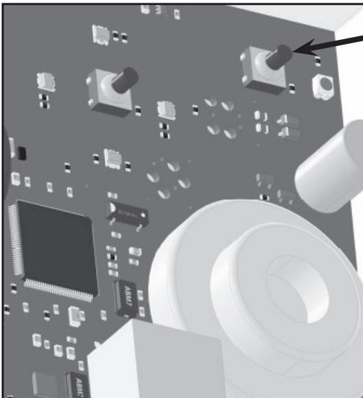
1. Press the Setup button on the Xpert Alert® WiFi alarm (the blue network status light will flash continuously).
