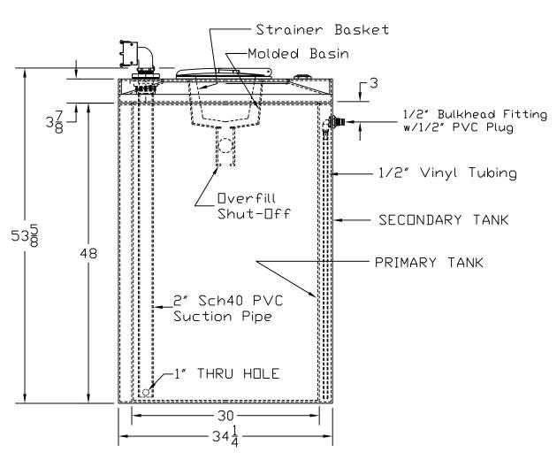
ALL DIMENSIONS SHOWN ARE OUTSIDE PART DIMENSIONS IN INCHES,AND VARY BY THE STANDARD ROTATIONAL MOLDING TOLERANCE OF 2% TO 3%.
