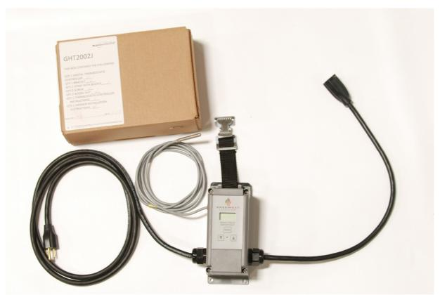
GHT2002J Thermostatic Controller. From left to right, please note the input power supply cord (~6' long) with plug, gray temperature sensor lead (~6' long) with steel encased temperature sensor/probe at the end, hanger kit installed and the output 2' long cord with connector (a k a receptacle).
