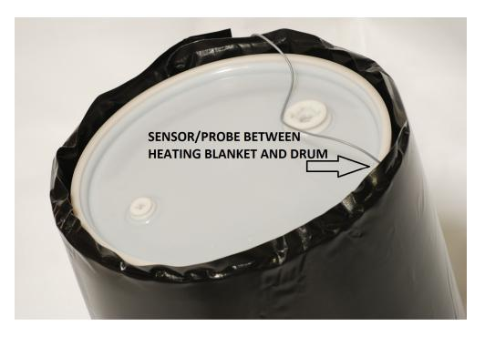
VERY IMPORTANT: Place the temperature sensor between the heating blanket and that which is to be heated, for example, your barrel or tote.
