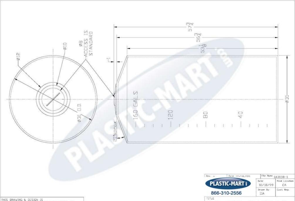
THE PROPERTY OF CHEM-TAINER INDUSTRIES INC. IT MAY NOT BE USED FOR ANY PURPOSE OTHER THAN BY THE OWNER. CHEM-TAINER DOES NOT ALL DIMENSIONS SHOWN ARE DUTSIDE PART DIMENSIONS IN INCHES, AUTHORIZE THE REPRODUCTION OR CONVEYANCE AND VARY BY THE STANDARD ROTATIONAL MOLDING TOLERANCE OF ±2%. OF ANY INFORMATION CONTAINED HEREIN.
